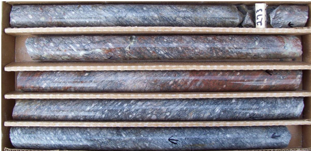
FIGURE 3.15 Drill core from the Leatherwood Granite showing highly sheared and mineralized granite. The average \text{U}_3\text{O}_8 percentage in this 10-foot core section is 0.679%. SOURCE: Wales (2010 49 ).
