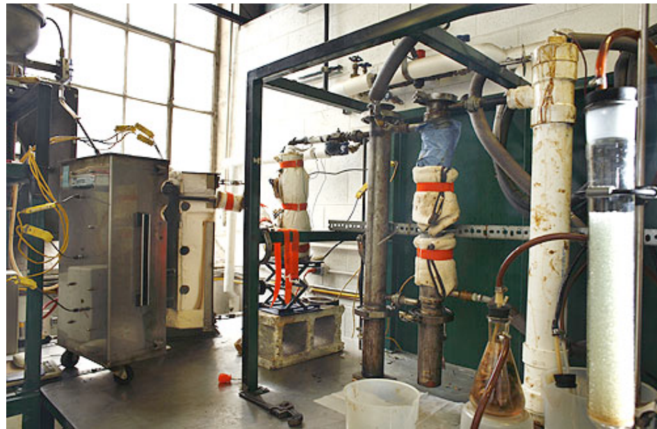
Bench-scale green diesel set-up in the Virginia Tech lab of Dr. Foster Agblevor.
