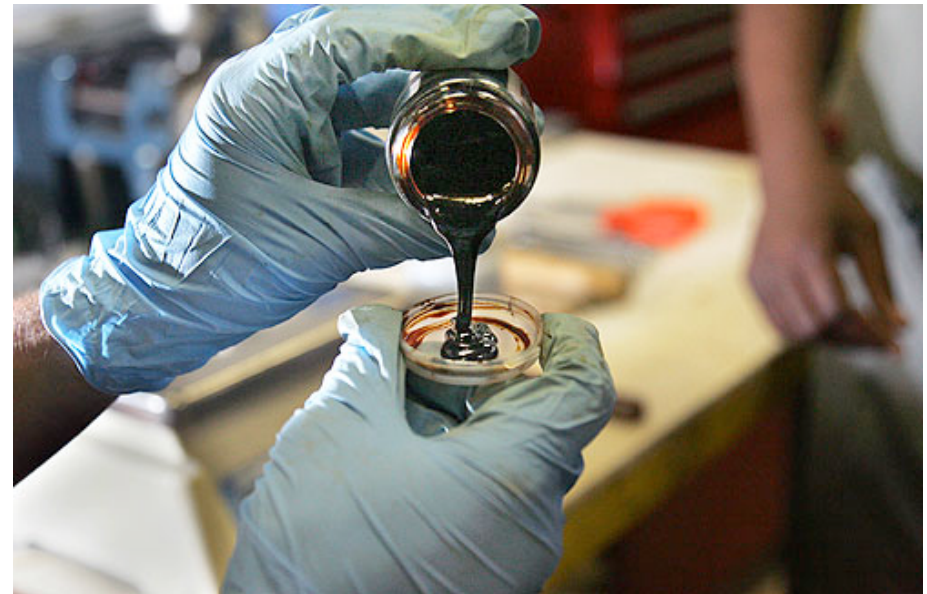
Pyrolysis oil, an intermediate product in the creation of green diesel, produced in Dr. Foster Agblevor's Seitz Hall laboratory.
