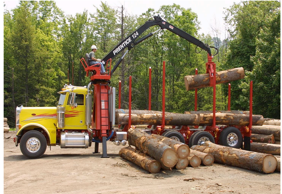
Mechanical grapping systems reduce loading labor costs by 50% and truck load time, thus increasing loads hauled per day, and decreasing feedstock costs.
